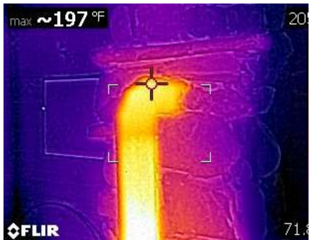
Figure 37 Thermal image of stovepipe in operation
